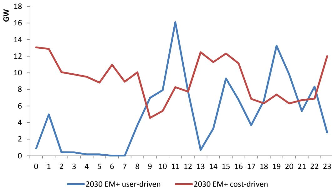
**Figure 3: Maximum EV charging power over 24 hours**
